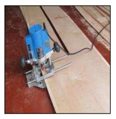
Then to save time and effort on fairing the hull at a later stage the edges are routed out to a shallow depth just sufficient to accept the tape
