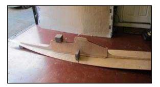
Finally the whole assembly is glued to the floor panels. I mounted it on a bench and working from below screwed it together first, took it apart, applied the epoxy glue, re screwed it and place it on a level floor to set: ensuring that the measurements from the base line were correct.
