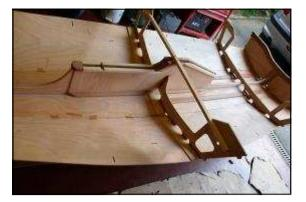
Some floor battens are inserted and glued as they are easier to reach now.
