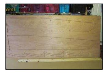
The ply sheets arrive, precut by router and are quickly and easily removed. I was amazed that within a couple of hours I had most of the parts ready to assemble. When I built 3838 it took me days to scale up the drawings onto ply sheets and cut out with a jig saw
