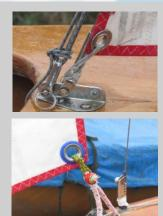
• Attach the jib sheets to the clew of the jib.
