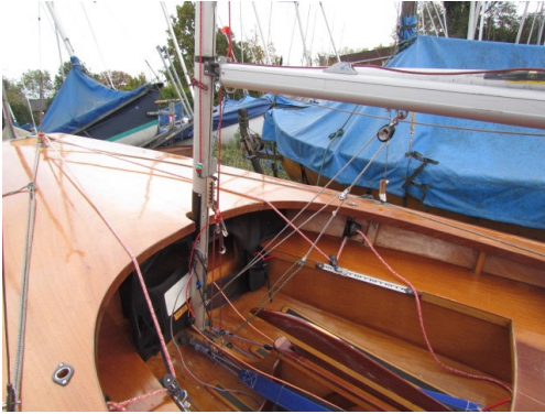
Detail of kicker and inboard sheeting
