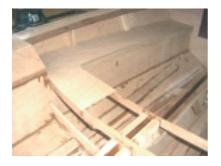
Extend the centre case ply upwards to place the new seat on shape and attach two lengths of the hardwood to form the base of the seat using epoxy glue
