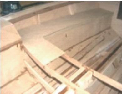
Extend the centre case ply upwards to place the new seat on shape and attach two lengths of the hardwood to form the base of the seat using epoxy glue
