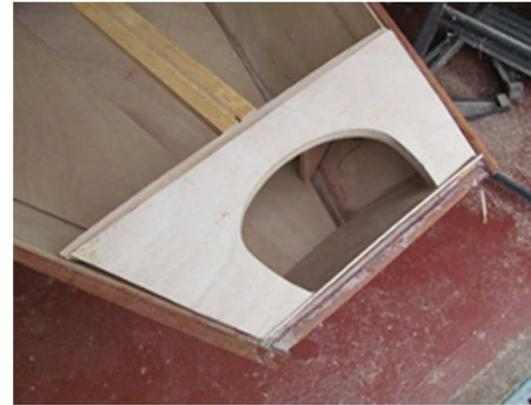
The components of the central chute can now be added, but oops Part 44Z is not exactly correct and I think I will have to add a bit of hardwood behind the mouth to provide a solid surface to screw the jib plate onto.
