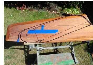
*Marking out the shape on the old centreboard. Blade is angled to make stronger use of the ply directions*
