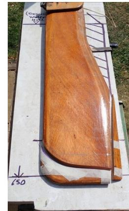
*Reshaping to reduce depth and tip area*
