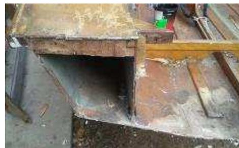
the new transom (including slot tabs to be on the safe side). A little tip when cutting ply, run masking tape along the pencil line so that when you cut with your jigsaw it does not splinter the wood. It works!
