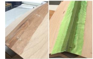
The outer chine which was laminated and finished with peel ply
