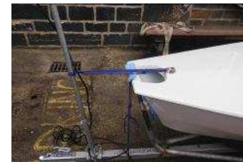
Bow tied to stop boat sliding back when being towed
