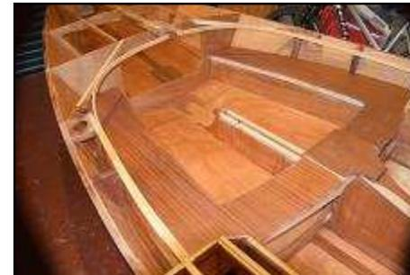
The last two pictures show the false floor, integral seat tops and thwart ply in position but yet to be glued and trimmed.
