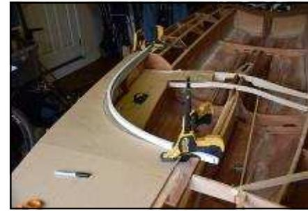
Cardboard templates are made for the deck panels, these are then cut out from two sheets of Tiger striped sapele along with the seat tank tops
